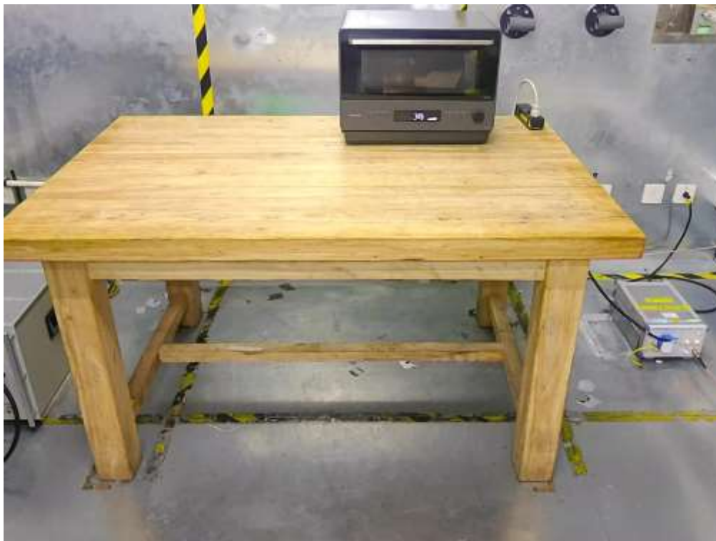
AC Power Line Conducted Emissions
