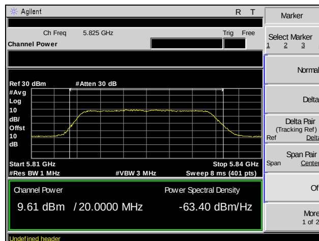
Plot 19. RF Power Output, Channel 165, 802.11a 20 MHz, MIMO
