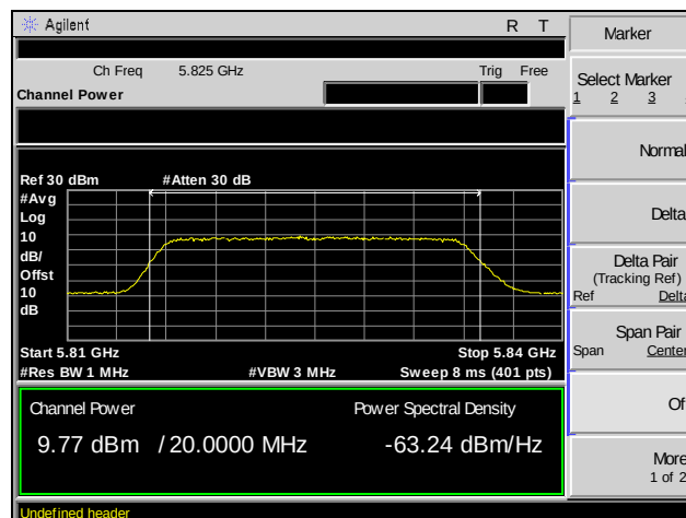
Plot 37. RF Power Output, Channel 165, 802.11n 20 MHz, MIMO
