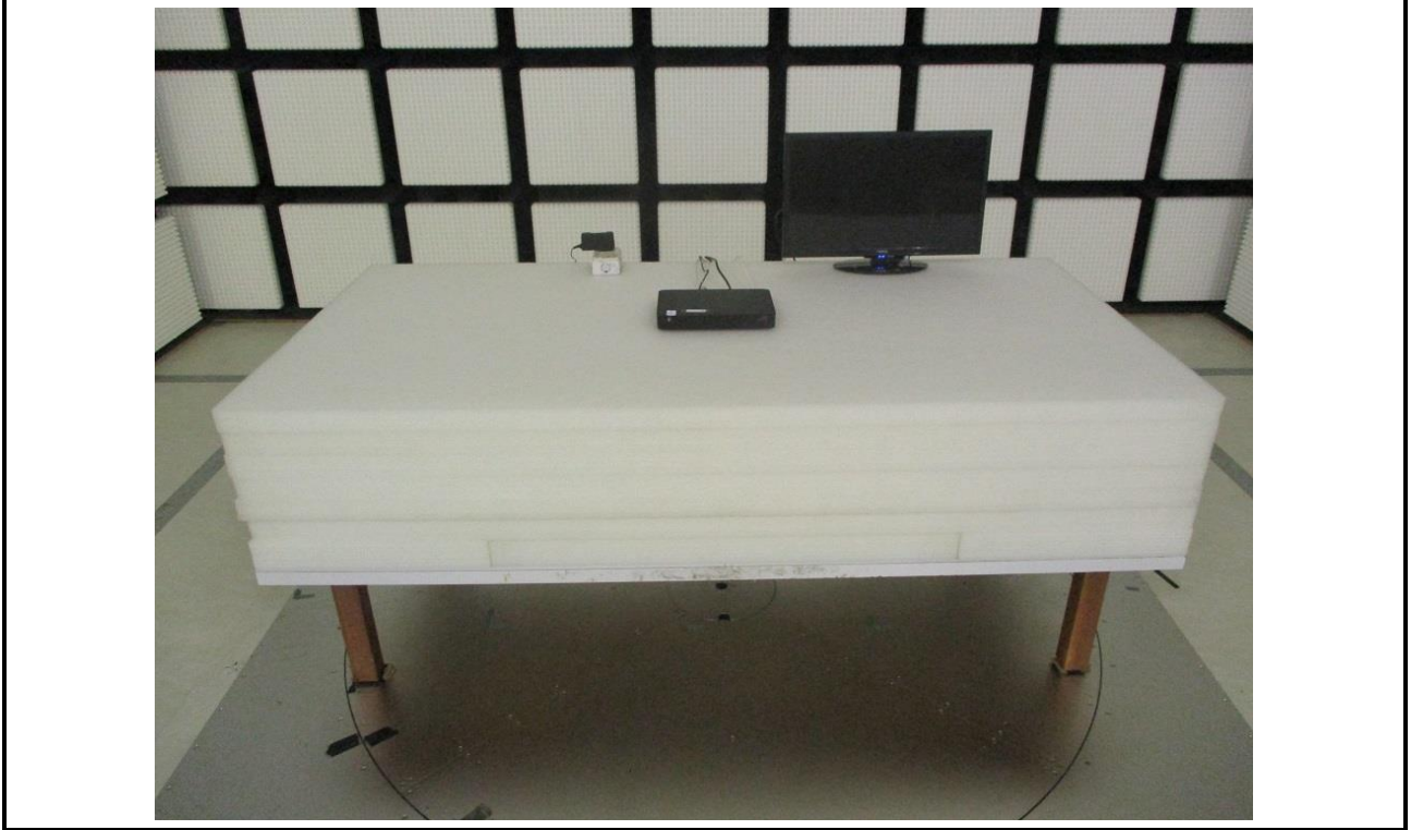
Radiated Emission Below 1GHz Test
