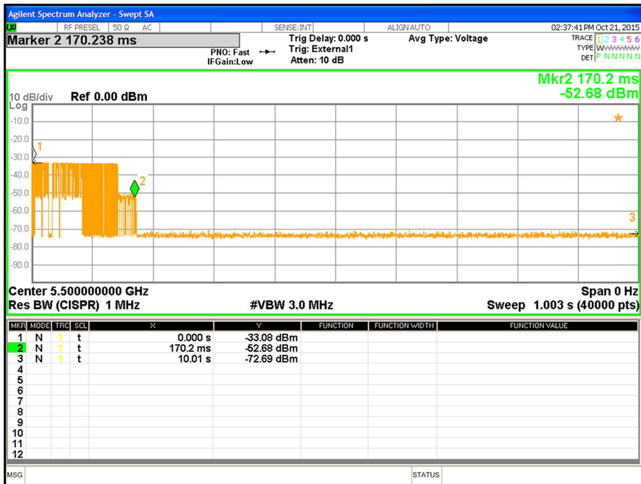
Figure 9: Channel moving time at 5500MHz Zoom in Plot _with 20MHz BW
