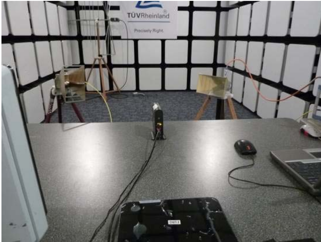
Figure 1: Dynamic Frequency Selection Test Setup – Rear View
