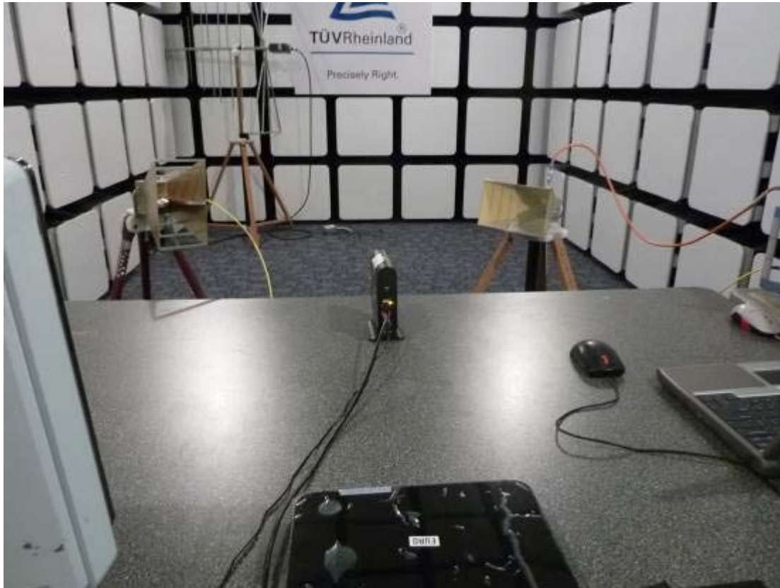
Figure 1: Dynamic Frequency Selection Test Setup – Rear View
