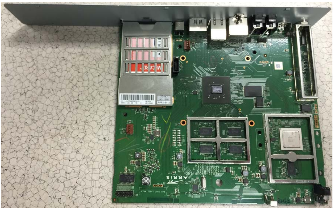
Top View Heat Sinks and Shields Removed
