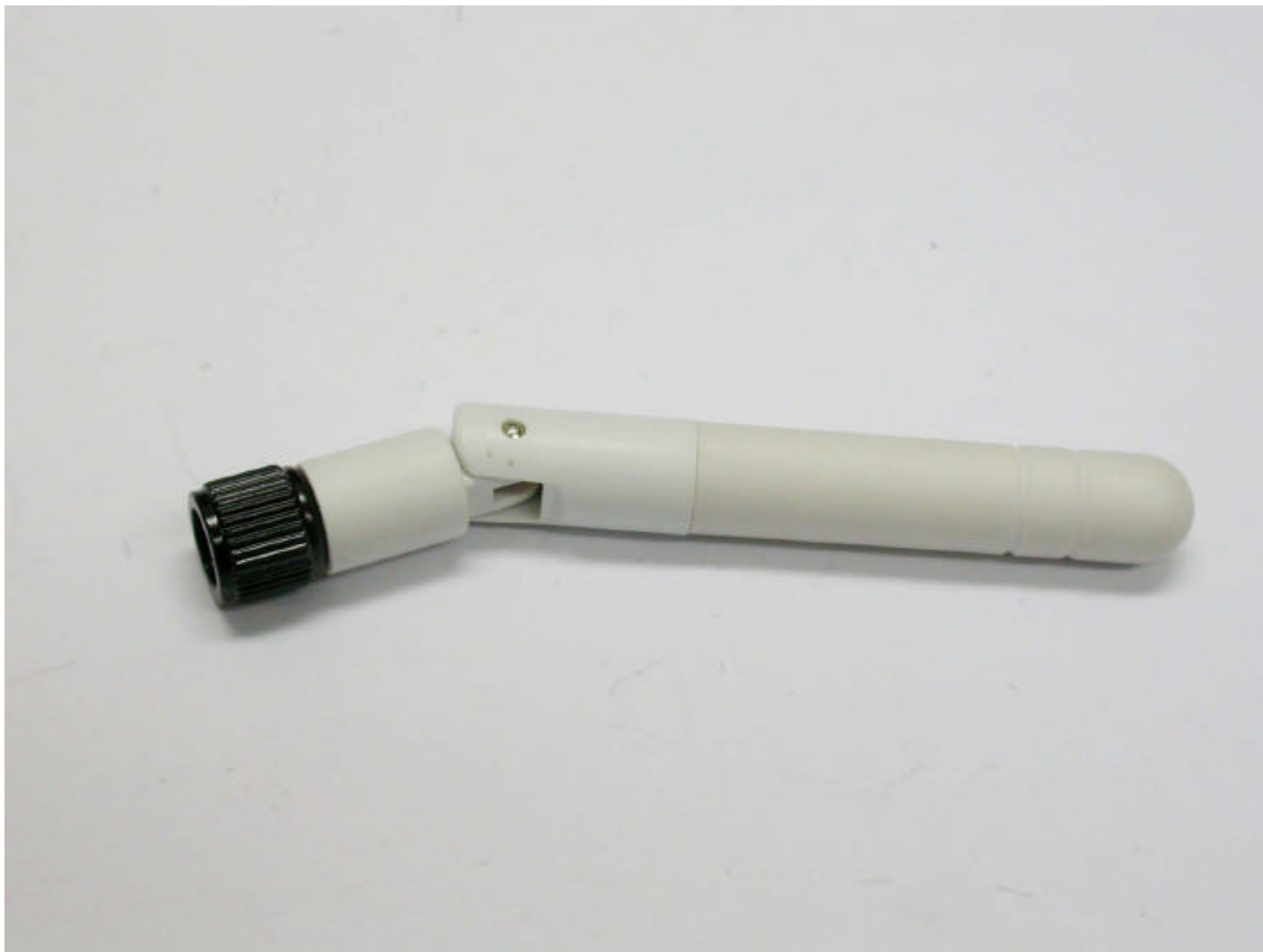
Antenna type 1: Reverse SMA connector, dipole antenna
