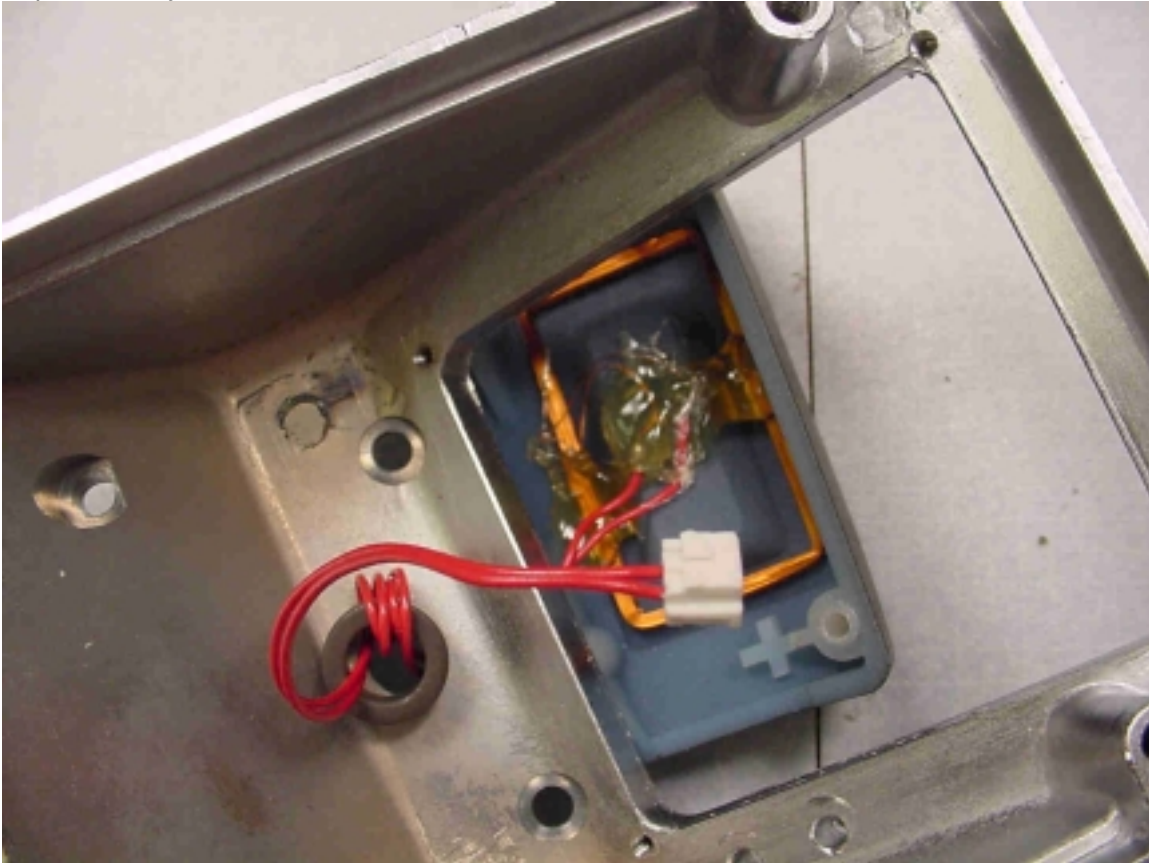
Antenna and leads viewed from inside the housing
