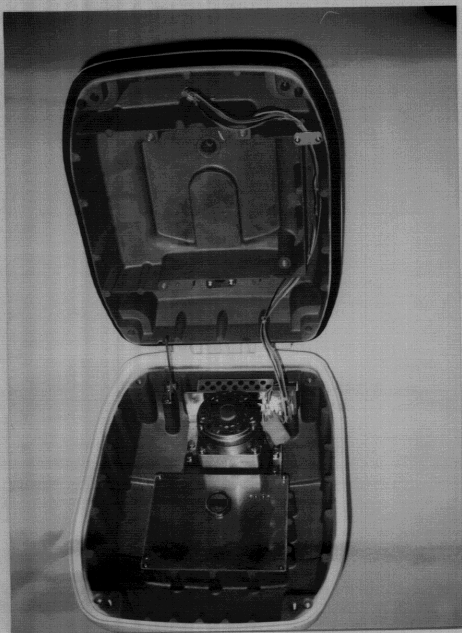
SCANNER UNIT INSIDE VIEW (RF MODULE REMOVED)
