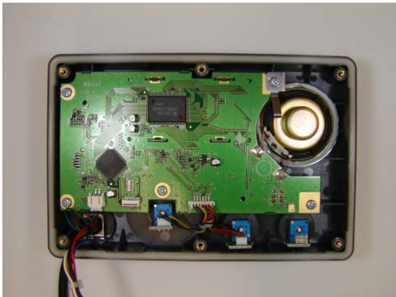
Front panel -inside view
