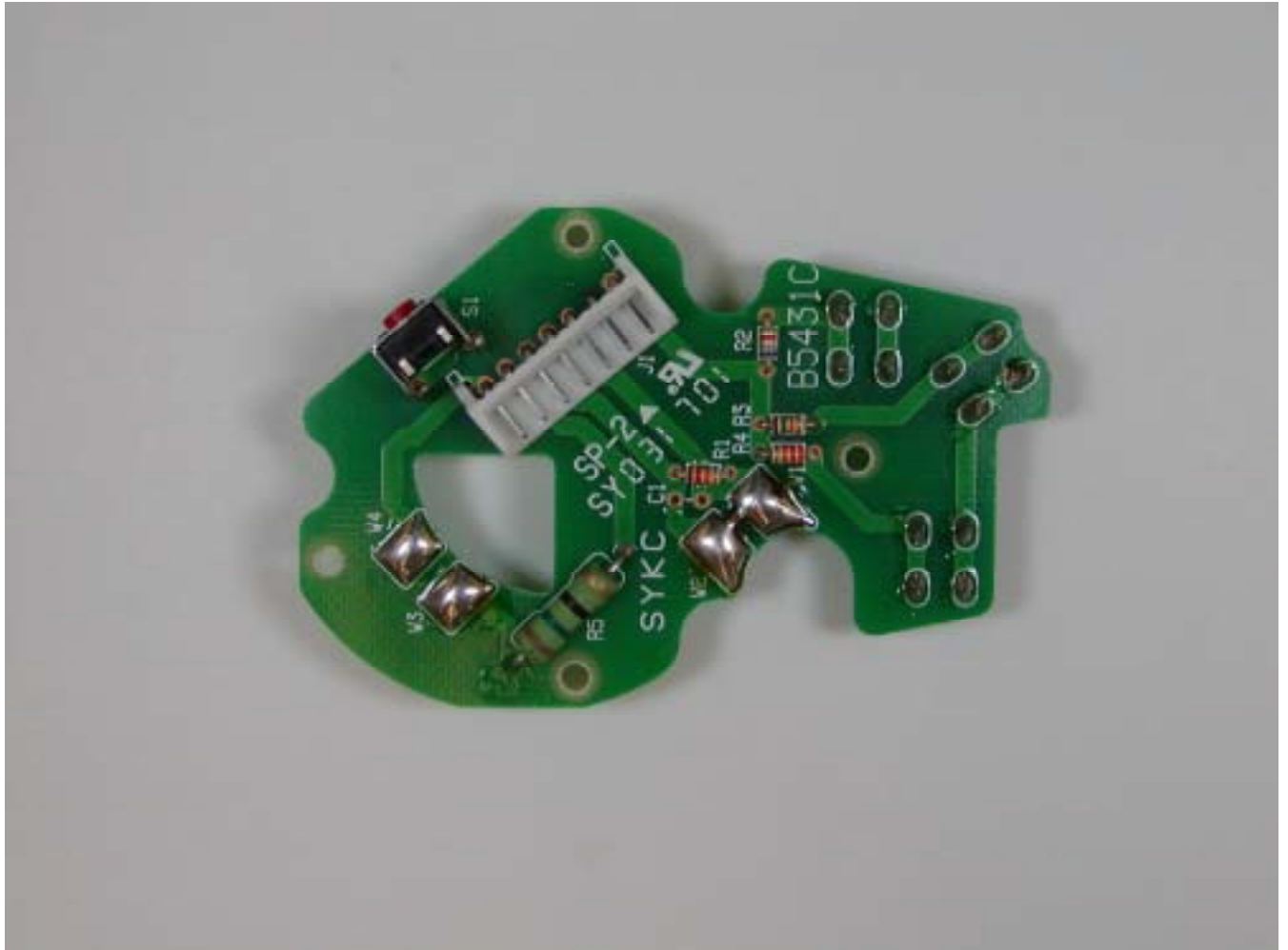
Microphone PCB - fron view
