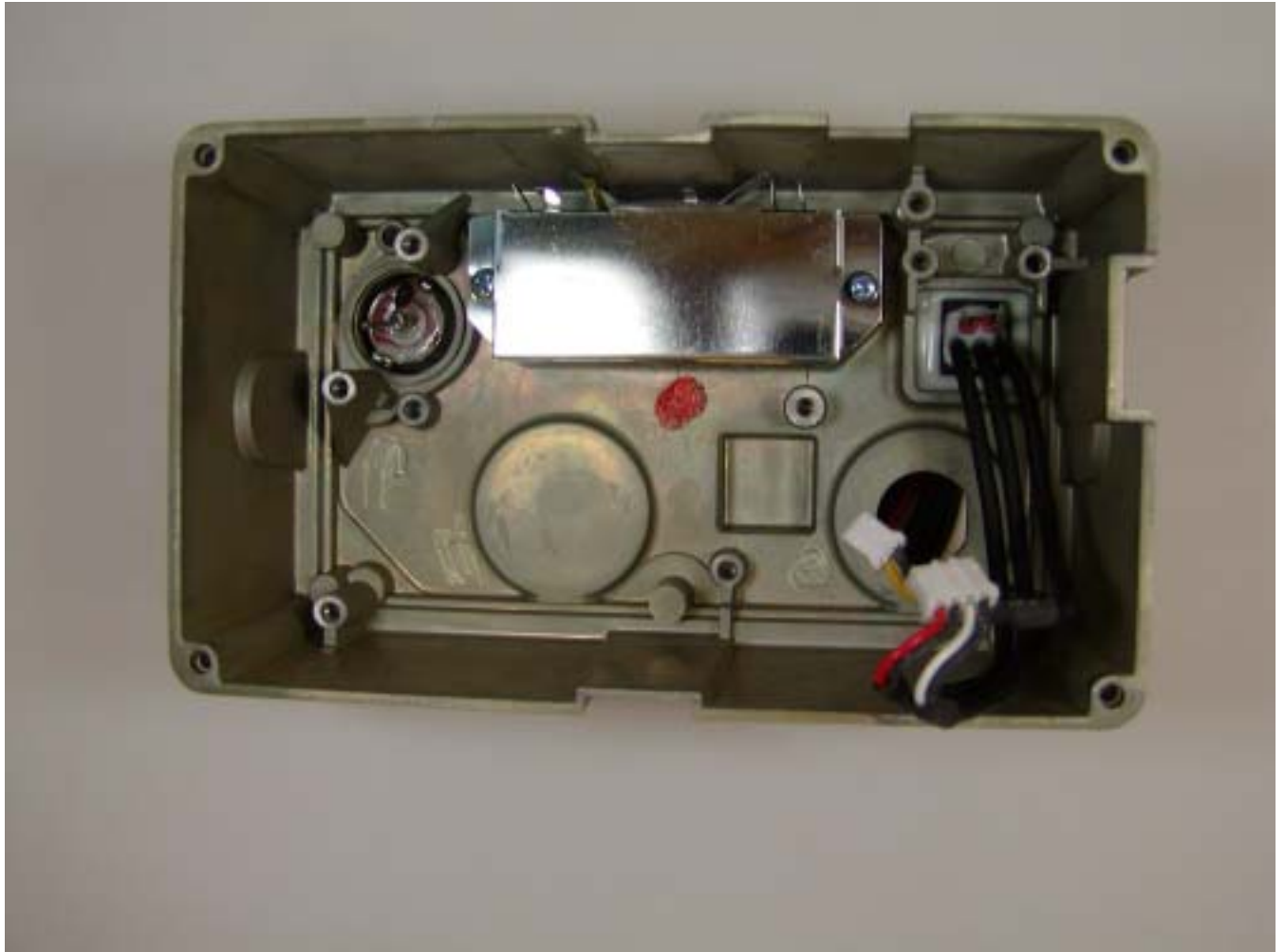
Rear chassis removing all PCBs
