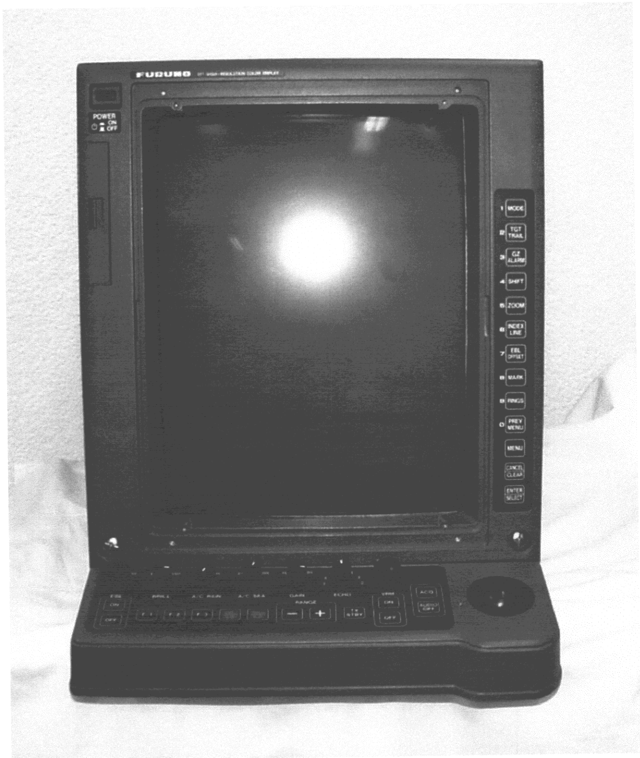
Photo 10.1 Display Unit (RDP-120) Front View
