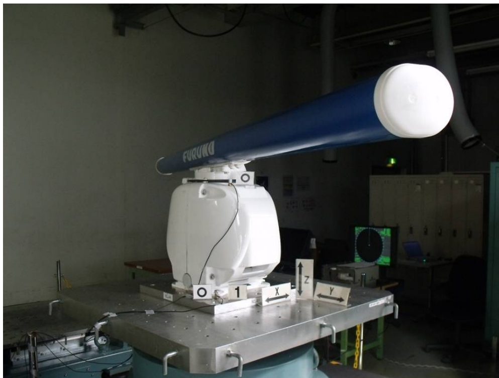
Antenna Unit (RSB-128 + RTR-106 + XN24CF),
