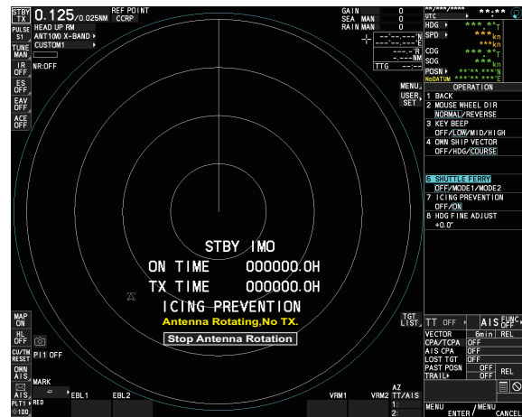
When the antenna rotates
