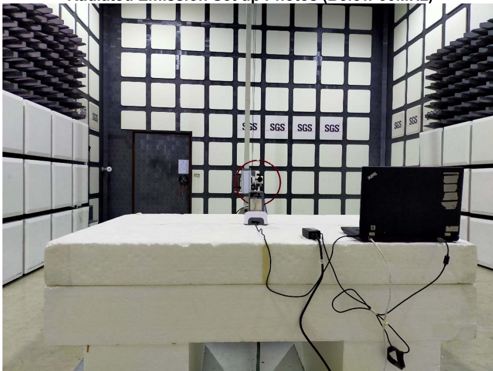
Radiated Emission Set up Photos (Below 1GHz)
