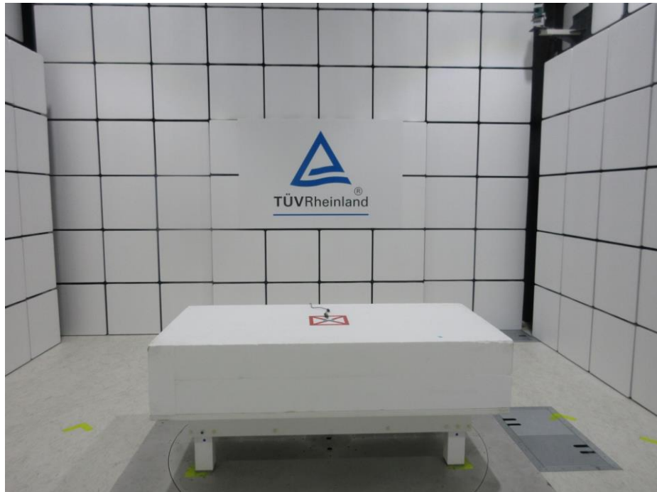
Photograph 1: Set-up for Spurious Emissions (Front View 1)
