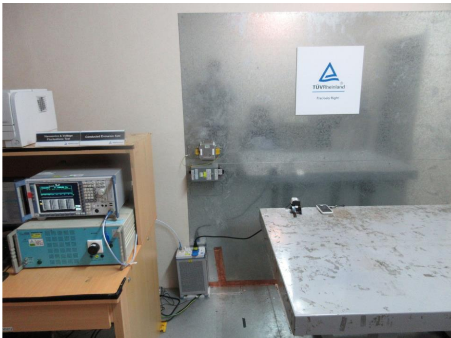
Photograph 4: Set-up for Mains Conducted testing (Front View)
