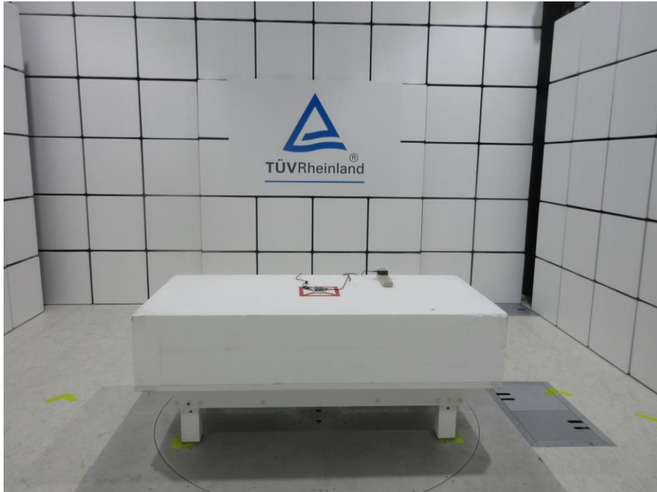
Photograph 1: Set-up for Spurious Emissions (Front View 1)
