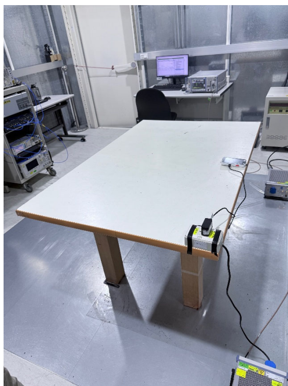
Back View of AC Power Line Conducted Emission Test
