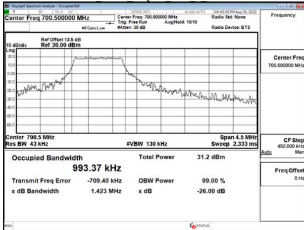
Band12 3MHz 16QAM RB5 0 CH23095
