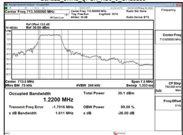
Band12 5MHz QPSK RB6 0 CH23155
