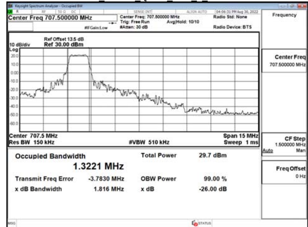
Band12 10MHz QPSK RB6 0 CH23130
