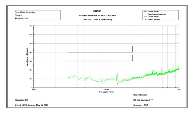
Intertek Radiated Emissions 30 MHz - 1000 MHz EN55022 Class B (QP-Horizontal)
