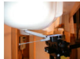
Figure 14.8 Right Head SAR Test Setup -- Ear / Tilt Position --
