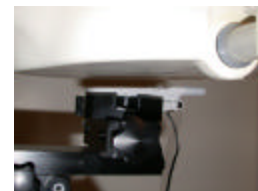
Figure 14.12 Body SAR Test Setup -- w/o Belt-clip --
