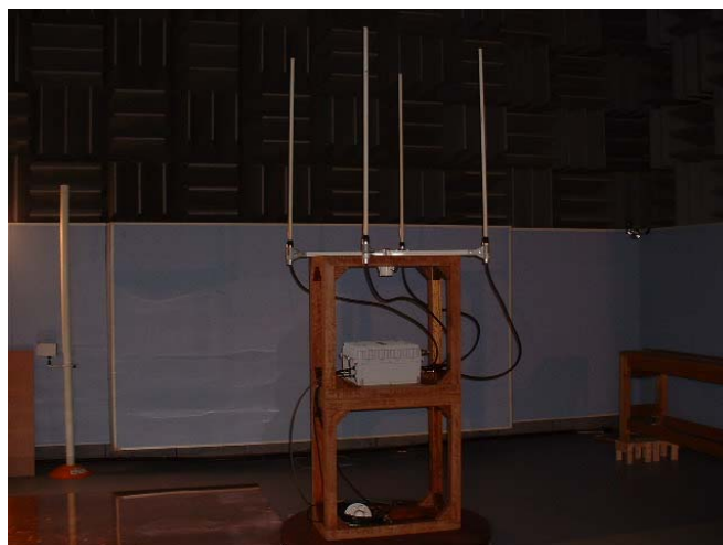
Side View(Transmitter Antenna System: ANT5-ANT8)
