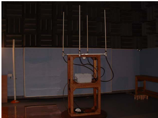
Side View(Transmitter Antenna System: ANT5-ANT8)
