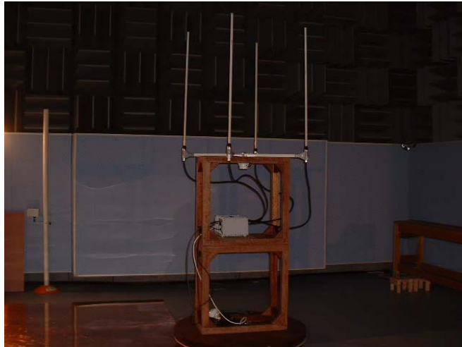
Side View(Transmitter Antenna System: ANT1-ANT4)
