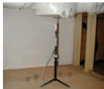
Figure 12.1 Dipole Validation Test Setup
