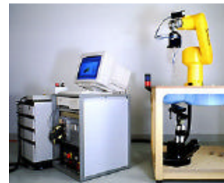
Fig. 1 SAR Test Setup
