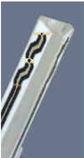
Figure 3.2 Probe Thick-Film Technique
