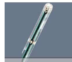
Figure 4 H-Field Free-space Probe
