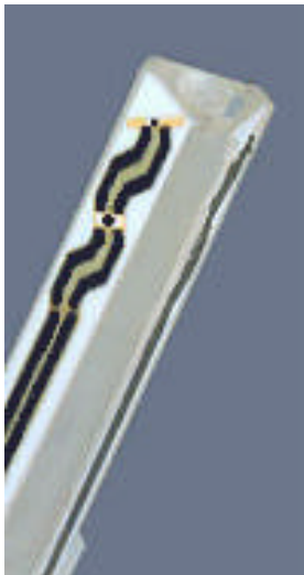
Fig. 5. ET3DV5 E-field Probe
