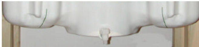
Figure 7.2 SAM Twin Phantom shell
