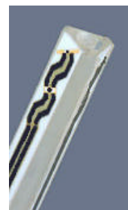
Figure 3.2 Probe Thick-Film Technique
