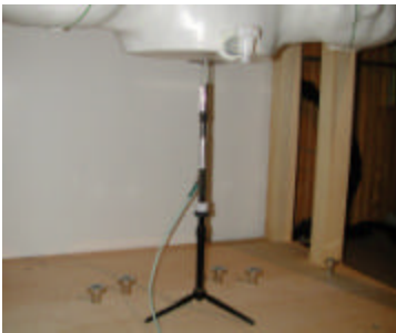
Figure 12.1 Dipole Validation Test Setup
