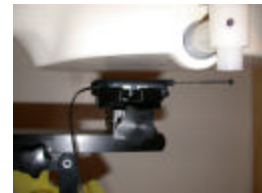
Figure 14.14 Body SAR Test Setup -- w/o Holster --
