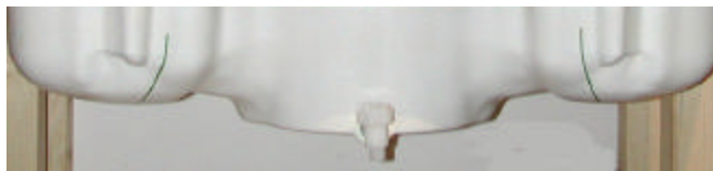
Figure 7.2 SAM Twin Phantom shell
