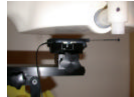
Figure 14.13 Body SAR Test Setup -- w/o Holster --
