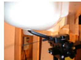
Figure 14.10 Right Head SAR Test Setup -- Ear / Tilt Position --
