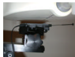
Figure 14.13 Body SAR Test Setup -- w/o Holster --
