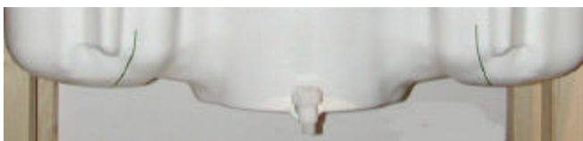
Figure 7.2 SAM Twin Phantom shell
