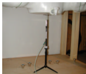
Figure 12.1 Dipole Validation Test Setup
