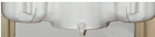
Figure 7.2 SAM Twin Phantom shell
