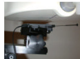
Figure 14.15 Body SAR Test Setup -- w/o Belt-clip --
