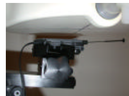
Figure 14.13 Body SAR Test Setup -- w/o Holster --
