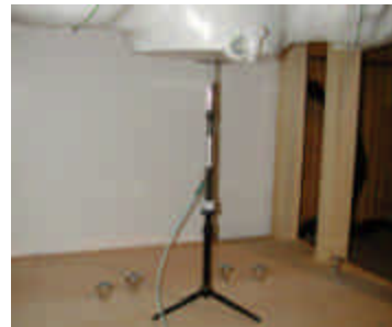
Figure 12.1 Dipole Validation Test Setup
