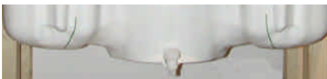
Figure 7.2 SAM Twin Phantom shell
