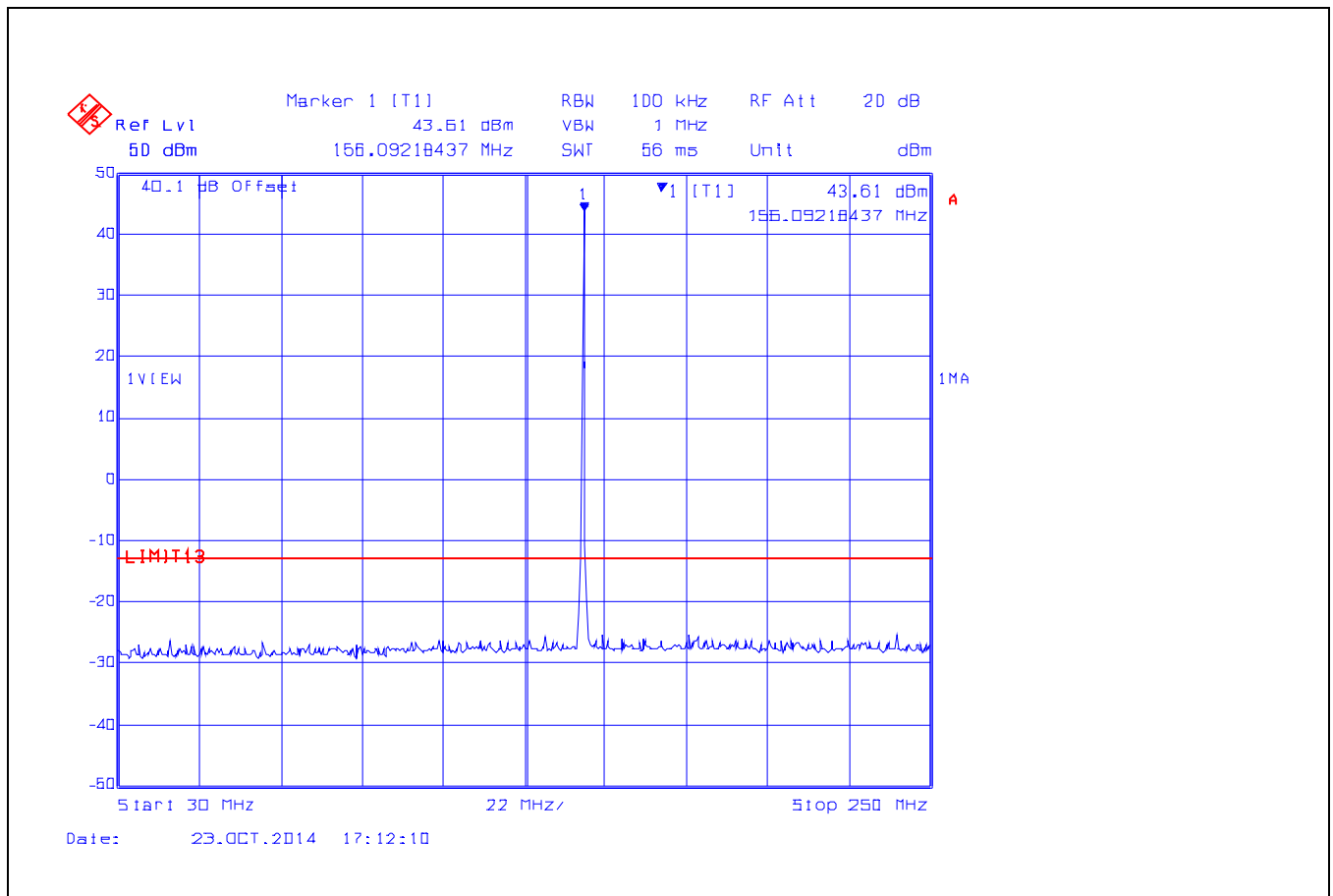
Plot 5.6.4.1. Spurious Emissions at Antenna Terminals, 156.050 MHz, 25 kHz Channel Spacing, 25 W, 30 MHz - 250 MHz
