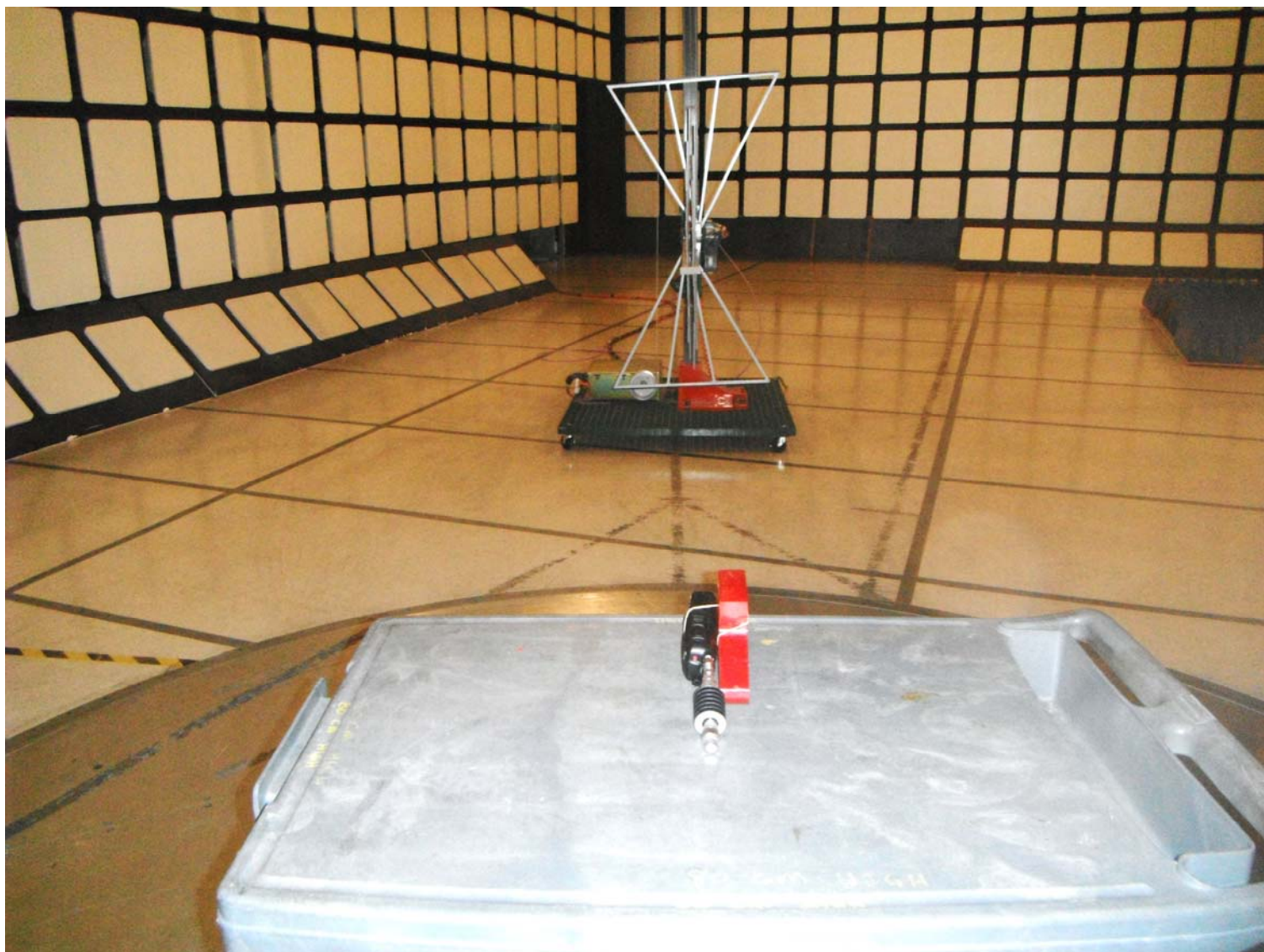
Plot #3: Tx Radiated Emission Test Setup
