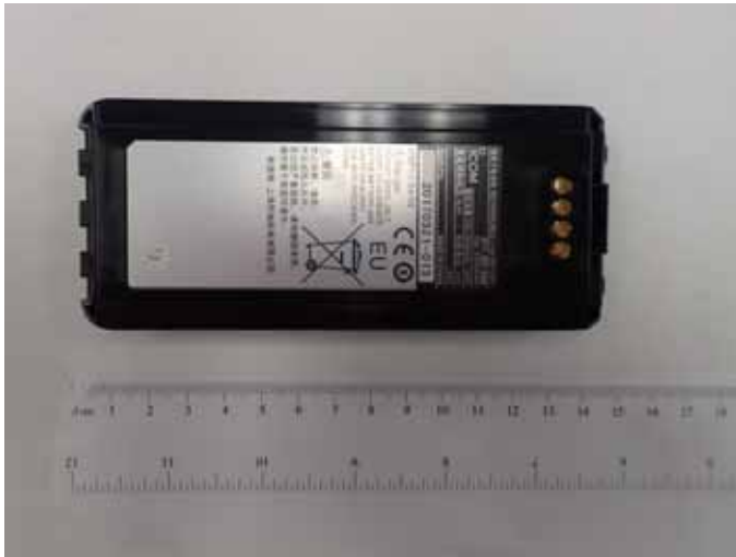
Li-ion Chargeable Battery (M/N: BP-288, 7.2V, 2350mAh)
