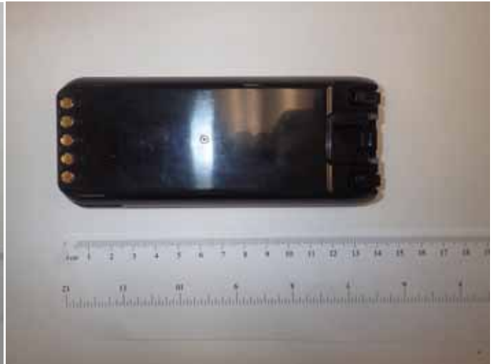
Li-ion Chargeable Battery (M/N: BP-288, 7.2V, 2350mAh)
