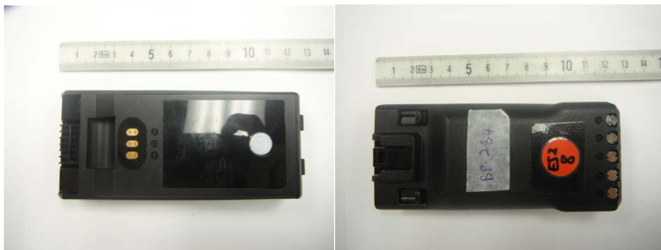
Li-ion Chargeable Battery (M/N: BP-285 Li-ion, 7.2V, 3210mAh)
