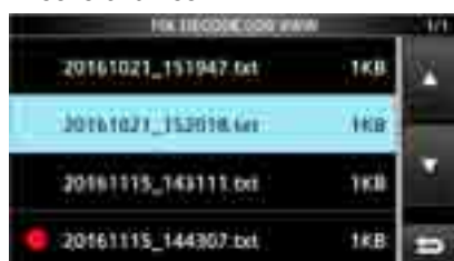
FSK DECODE LOG VIEW screen
