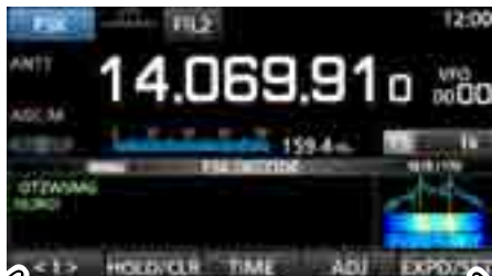
FSK DECODE screen
