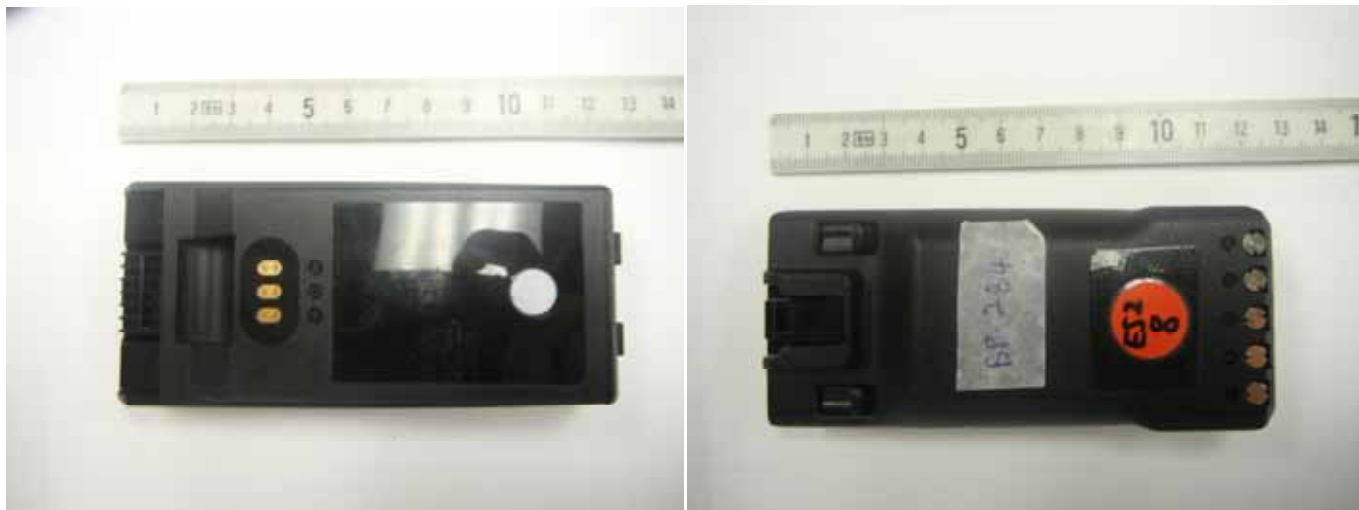
Li-ion Chargeable Battery (M/N: BP-284 Li-ion, 7.2V, 3210mAh)
