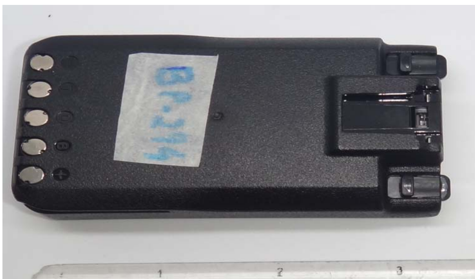
Li-ion Chargeable Battery (M/N: BP-294 Li-ion, V, 1960mAh)
