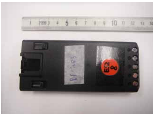
Li-ion Chargeable Battery (M/N: BP-283 Li-ion, 7.2V, 2010mAh)
