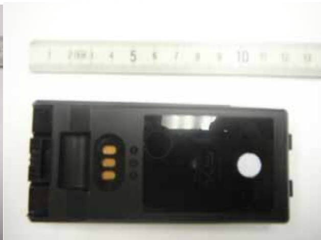
Li-ion Chargeable Battery (M/N: BP-283 Li-ion, 7.2V, 2010mAh)
