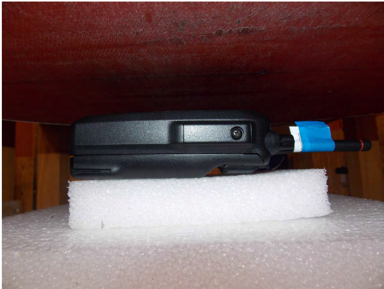
Test Position Face 25 mm Gap
