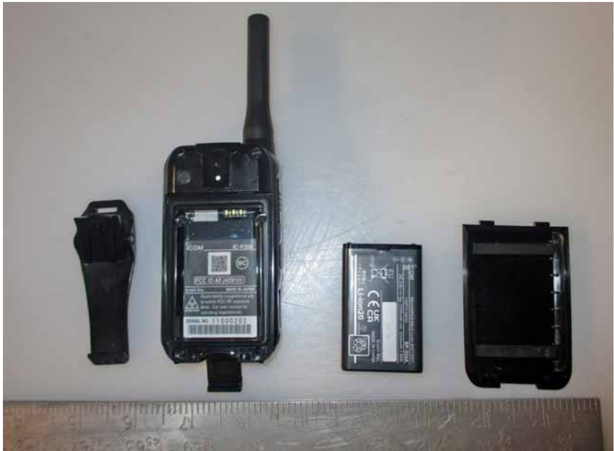
IC-F200 Rear Side with cover battery belt clip removed
