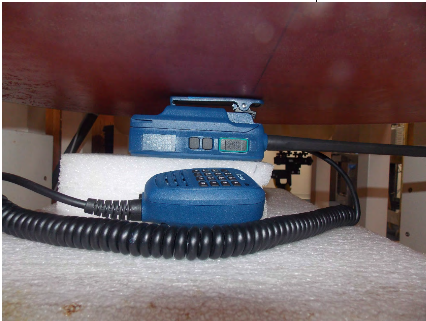
Handset with Antenna C, Audio A and Body A 0 mm Gap Accessories Configuration
