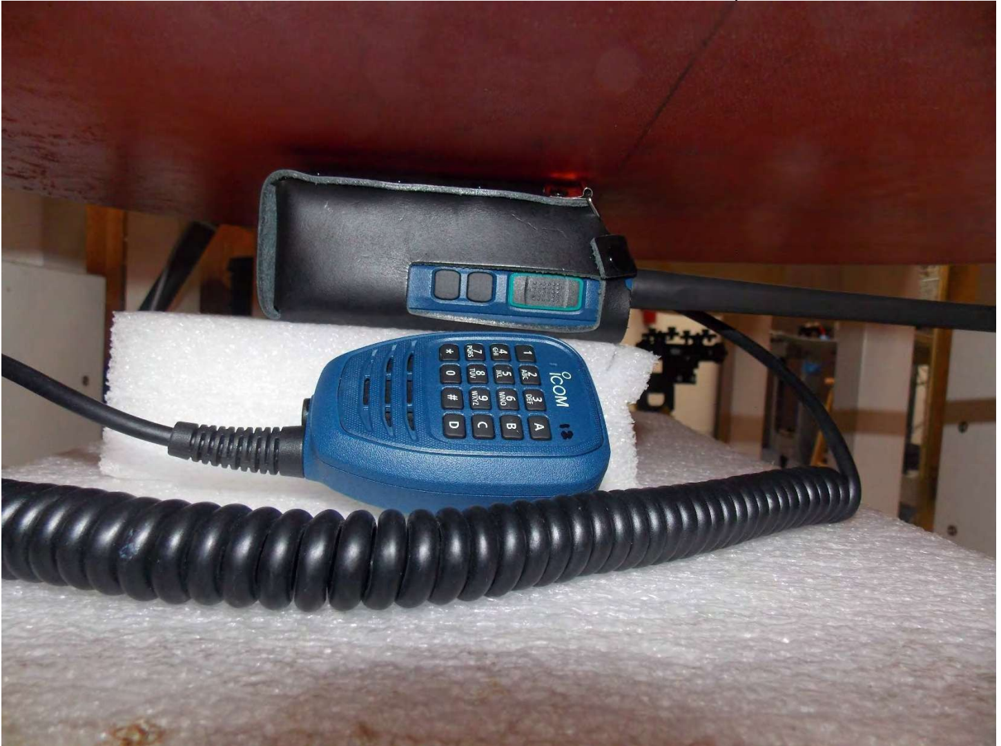
Handset with Antenna C, Audio A and Body B Accessories 0 mm Gap Configuration
