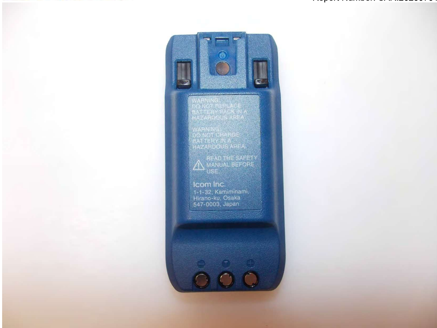
Back of Battery
