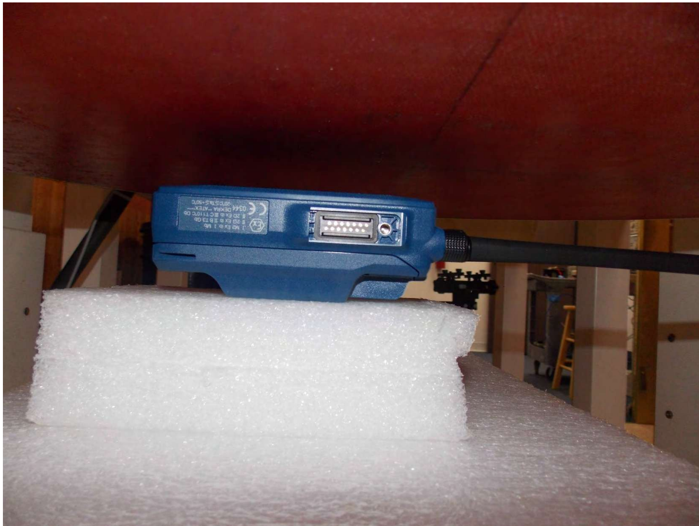
Handset Face Ant C 25 mm Gap Configuration
