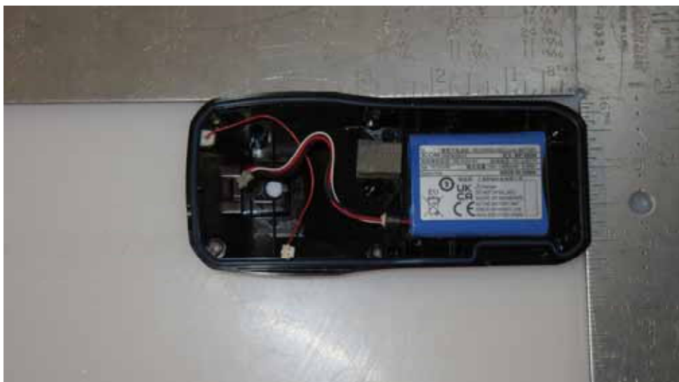
<Li-ion Chargeable Battery (BP-282N, 3.6V, 1570mAh)>
