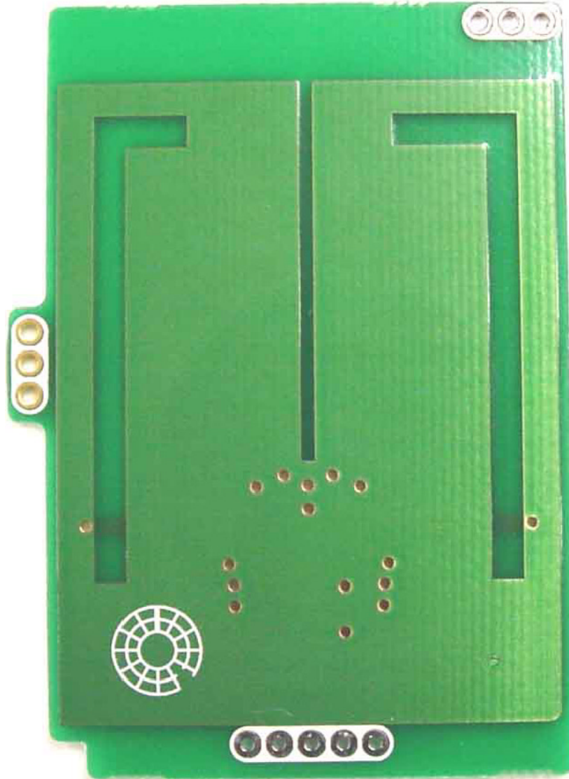
PHOTOGRAPH 9: TOP VIEW OF ANTENNA
