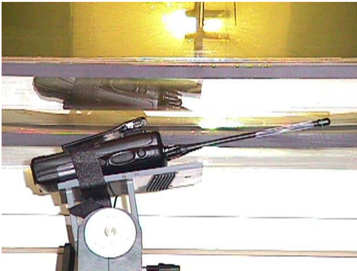
< The tip of the antenna in contact with the phantom with the alligator belt clip(M/N: MB-74) and headset(M/N: HS-51) – Close-up View >
